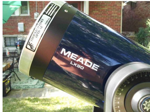
My 8-inch LX-90 Schmidt-Cassegrain telescope outfitted with a Thousand Oaks white light solar filter. Photo by Bill Breeden.
