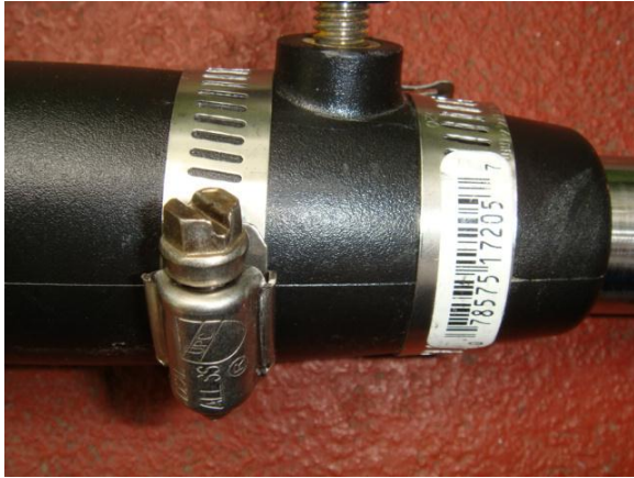
Fig. 2: The thumbscrews were removed from each ferrule to allow the cracked plastic to return to the un-tensioned position. Hose clamps were then positioned above and below the threaded bushing of each ferrule and firmly tightened. Photo by Mike Veith.
