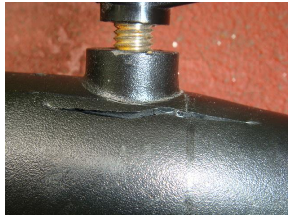
Fig.1. The plastic ferrule was cracked on both sides of the threaded bushing, through which the thumbscrew passes. Photo by Mike Veith.
