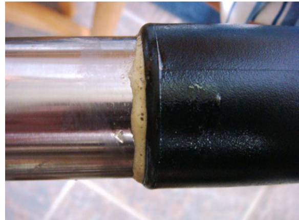
Fig. 3: A moist cloth was used to wipe off the excess glue as it expanded out of the ferrule to leave a thin, exposed bead. Photo by Mike Veith.
