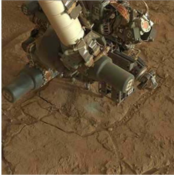
Curiosity performs series of tests with the robotic arm on a rock nicknamed "John Klein" to prepare for the first drilling to collect a sample of rock material on Mars.
