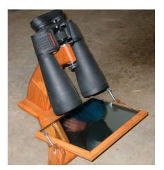
This homemade binocular viewer is the work of craftsman/astronomer Lee Paul. Total cost of the materials was about \$100. The mirror is "first surface," meaning that the top of the glass is silvered rather than the bottom as in a typical mirror. Now Lee can stargaze, shave and comb his hair at the same time.
